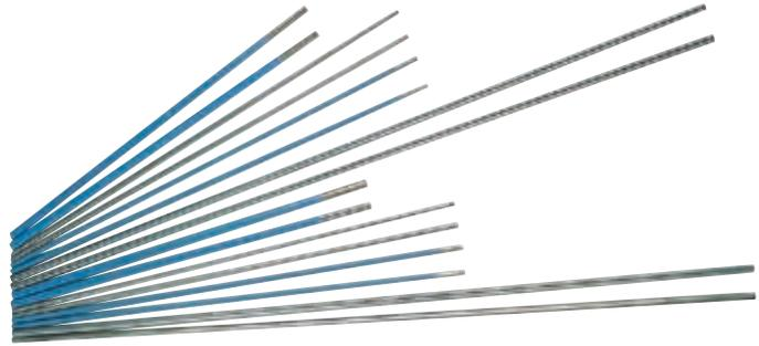
Unlike any other cutting process used today, the Arcair® SLICE systems can cut, burn or pierce virtually any metallic, non-metallic or composite material. Specially designed flux coated cutting rod, patented single piece construction maintains the balance necessary to sustain the exothermic reaction.
