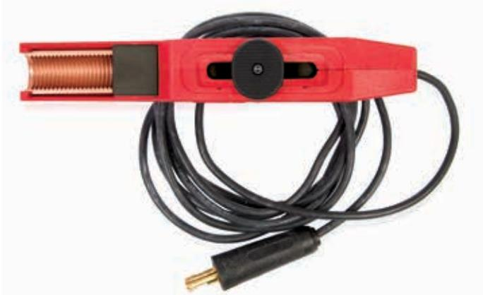
The SLICE Striker comes standard with a #10 AWG Power Cable with a twist-lock brass pin that can connect to the SLICE battery ignition source. The same twist-lock pin can be inserted into the mating receptacle on a plier type clamp found in the SLICE Utility Pack (please see separate fact sheet for details).
