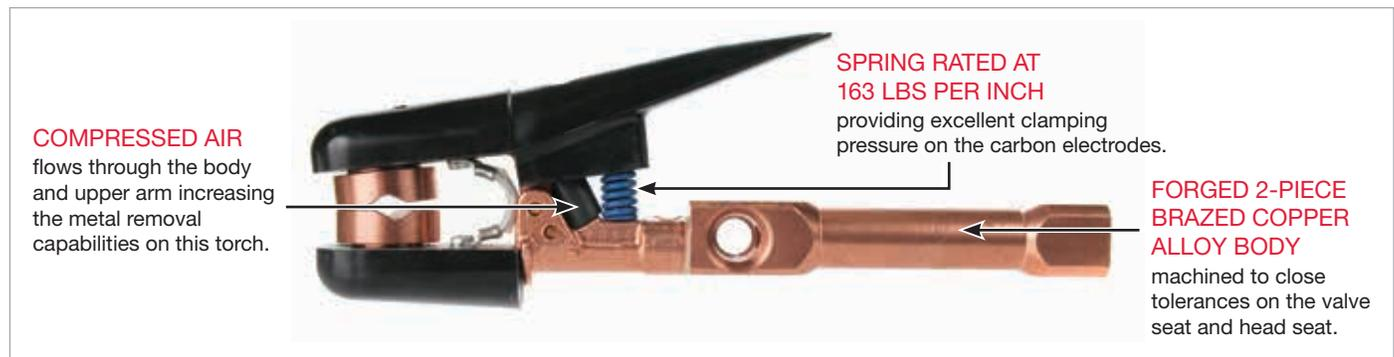
COMPRESSED AIR flows through the body and upper arm increasing the metal removal capabilities on this torch.
